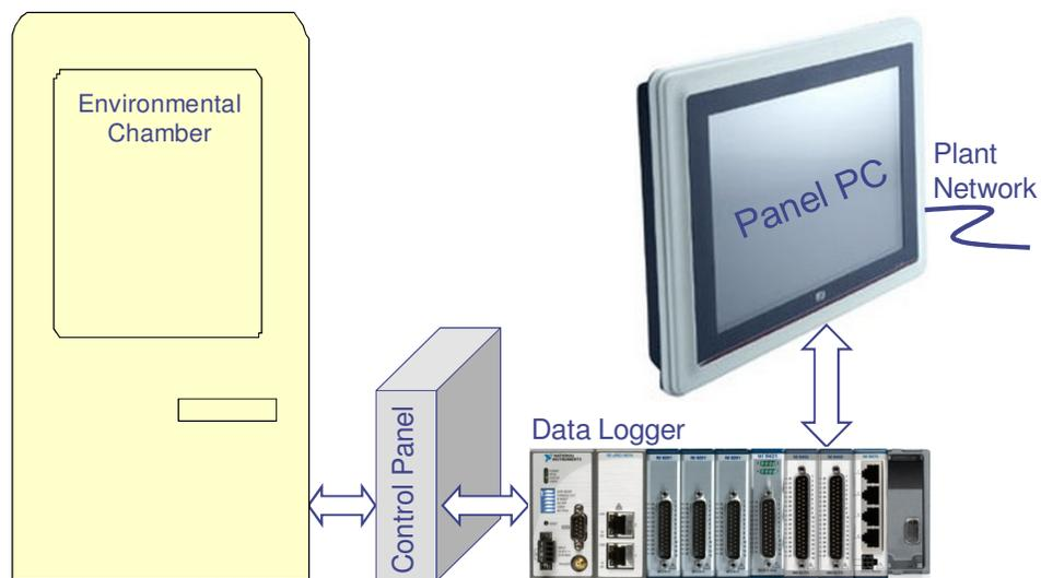
Figure 1. Environmental Test System Components and connectivity
