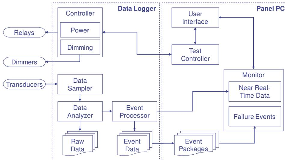
Figure 2. Environmental Test System Block Diagram
